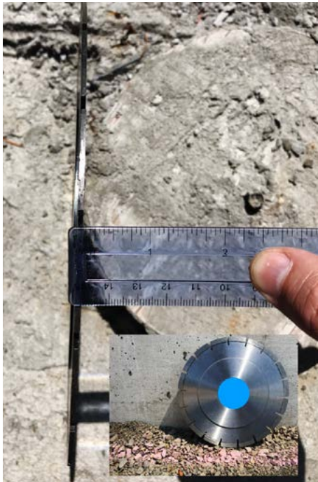
Using thin or “skinny” blades (1.6 mm [ \frac{1}{16} in.] thickness) reduces joint failure, spall, and maintenance throughout a facility’s life cycle. Creating thinner control joints also means using half the amount of filler materials than the older 3-mm ( \frac{1}{8} -in.) wide joints during initial construction.
