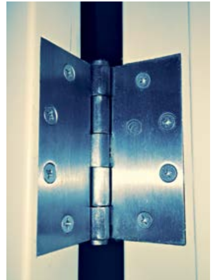
A five-knuckle non-bearing hinge is one of the most commonly used hanging devices, along with the bearing five-knuckle hinge. Non-bearing hinges allow the knuckles to rub together, causing wear of the metal over time, while bearing hinges allow for a smoother operation and less friction.
