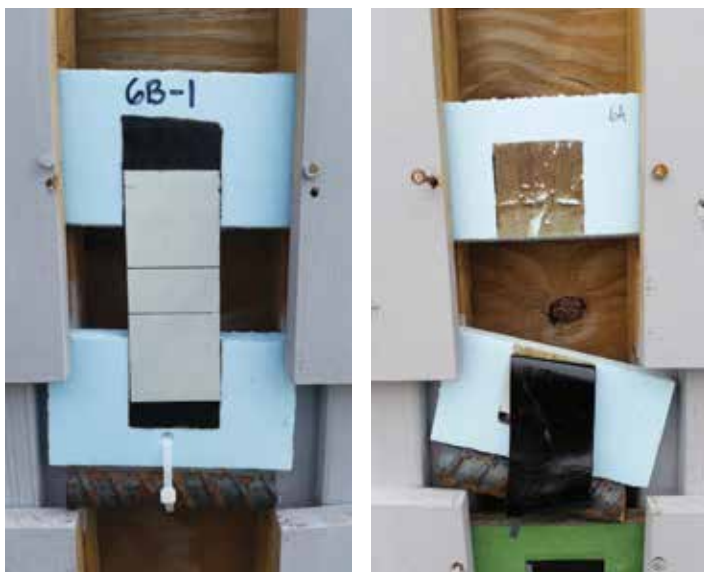
As illustrated by the photos above, the failure modes include vertical sliding and complete disbonding of the adhesive.
