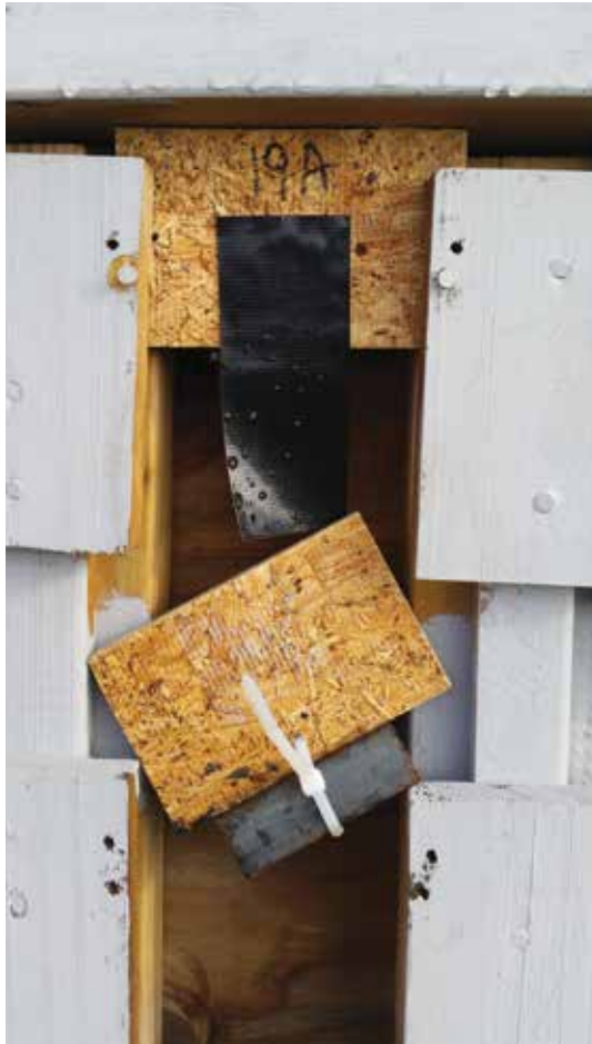
An example of tape failure.
