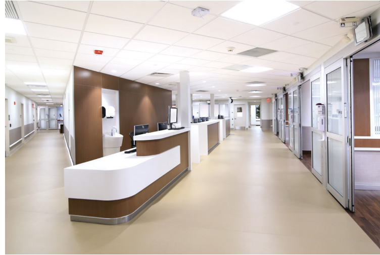
Fusion-bonded resilient flooring consists of a vinyl surface bonded to a vulcanized rubber performance backing to offer the hygienic benefits of hard surfaces with the acoustic and ergonomic traits usually associated with carpets and other textile flooring.
